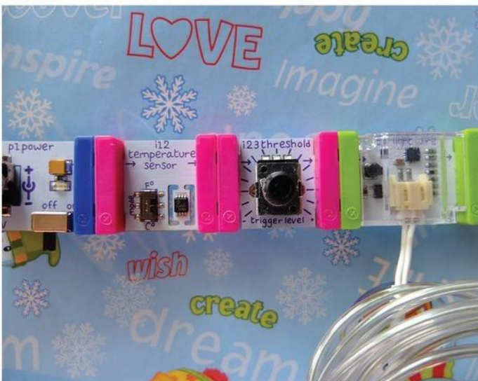
■ FIGURE 1. This wreath is triggered by temperature.
